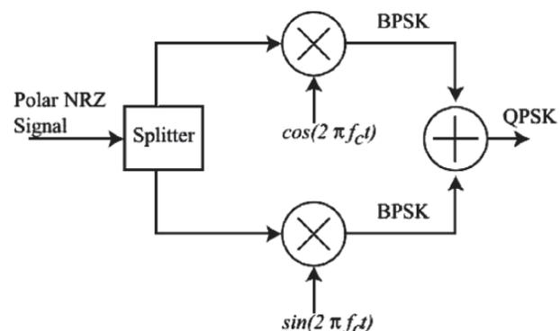
**Figure 7:** Generation of QPSK signal from polar NRZ signals
