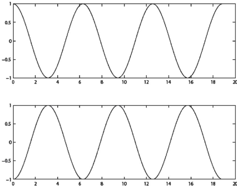
Figure 3: Signal set for BPSK with  $A = 1$
