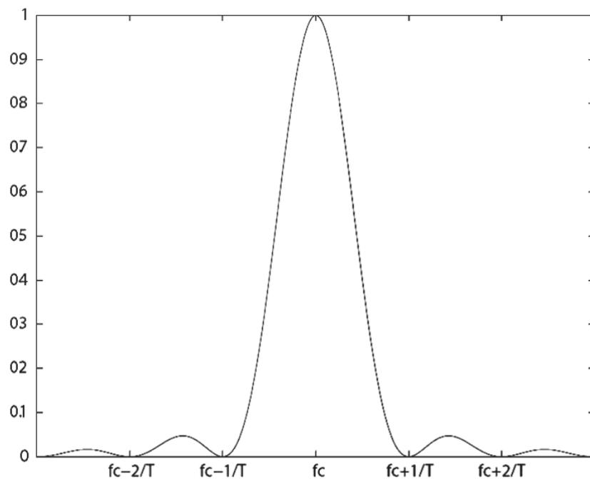
**Figure 10:** Power spectral density of BPSK signals
