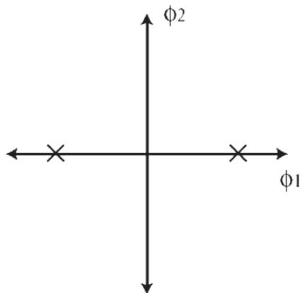
Figure 2: Constellation diagram for BPSK
