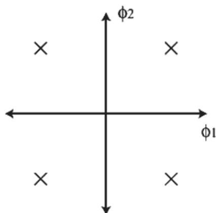
**Figure 6:** Constellation diagram for QPSK
