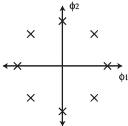
Figure 8: Constellation diagram for M-ary PSK
