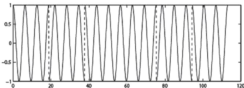
Figure 5: BPSK-transmitted signal for bit sequence 101101
